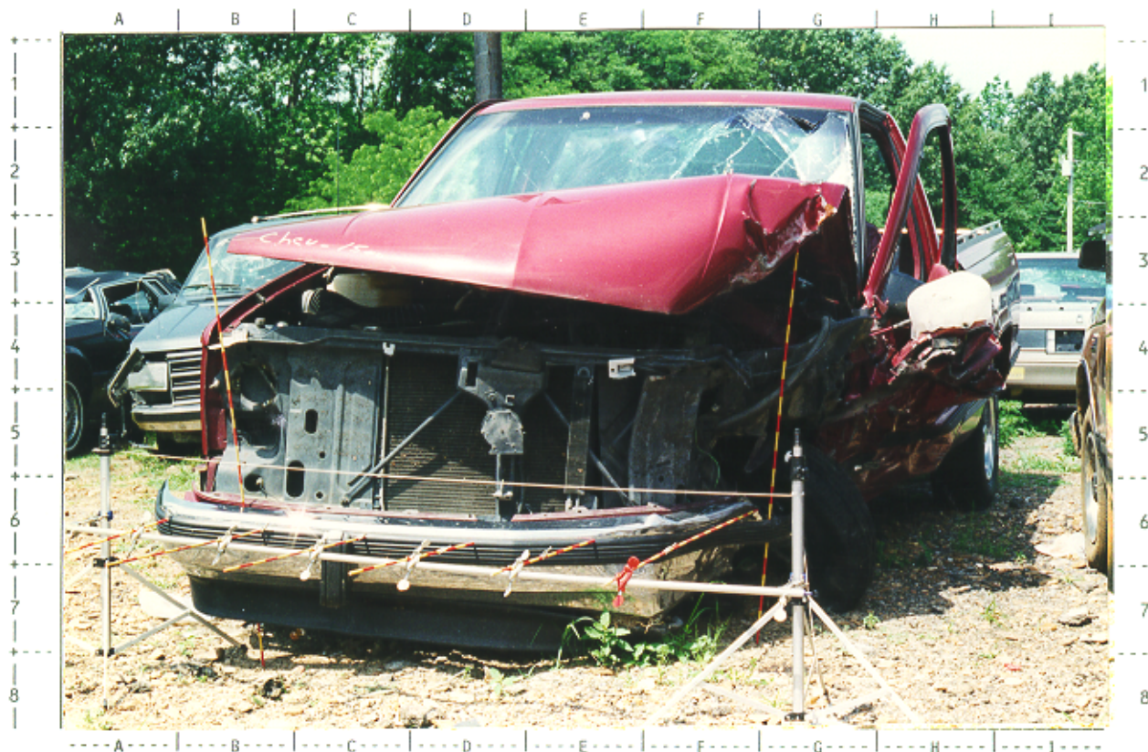
# 63 -- Front left view of '88 Chevrolet pickup's front left damage with contour gauge present; NOTE: FL hood damage and vertical rod
